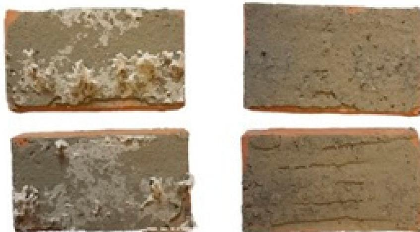
**Figure 6.** Surfaces of cement mortar glued to EPS (left—white, right—grey).
