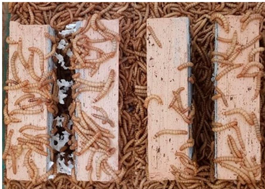
**Figure 5.** Specimens at the end of the experiment (left—with white EPS, right—with grey EPS).
